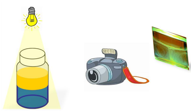
Figure S1. The illustration of setup used to record the evolution process of precipitation.
