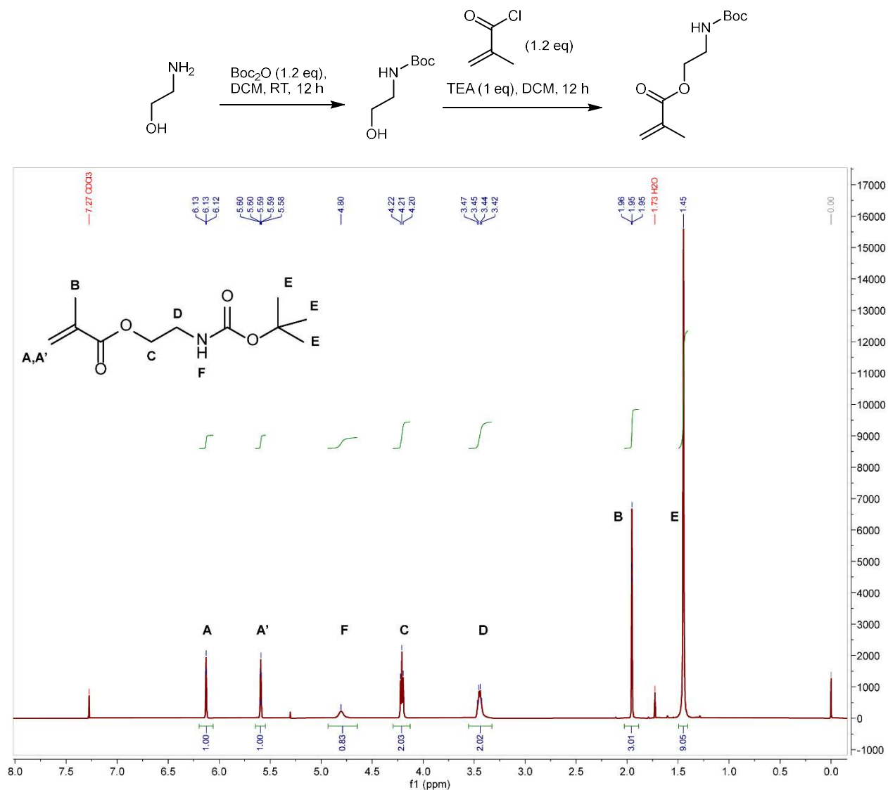
Figure S1: Synthesis of 2-(N-(tert-butoxycarbonyl)amino)ethyl methacrylate. Synthetic scheme and 1 H-NMR of 2-(N-(tert-butoxycarbonyl)amino)ethyl methacrylate (BocAEMA) in CDCl 3 at 400 MHz.
