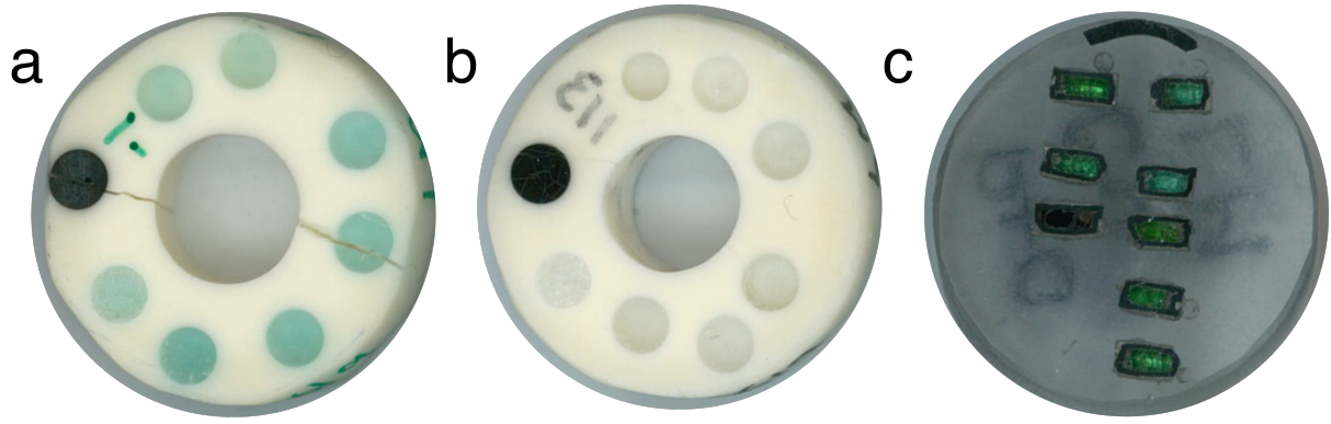
Fig. S1 Optical images of one MORB (black) and seven CMAS glasses equilibrated in (a,b) wells drilled in 25 mm diameter \text{Al}_2\text{O}_3 disks at (a) 1 atmosphere, 1300 °C, and \log f\text{O}_2 = -1 ( \Delta\text{QFM} = 7.3 ), (b) 1 atmosphere, 1300 °C, and \log f\text{O}_2 = -7 ( \Delta\text{QFM} = 0.3 ), and (c) Pt capsules at 1.0 GPa, 1400 °C and \log f\text{O}_2 = 4.8 ( \Delta\text{QFM} = 11 ), mounted and sectioned in epoxy.
