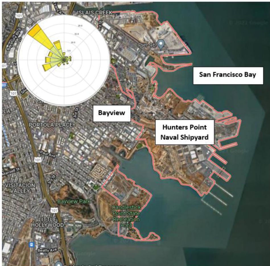
Figure 15. Wind rose depicting data collected at HPNS from 2005 to 2012. These data show that the wind blows predominantly away from the Bayview Hunters Point community and toward the San Francisco Bay. The spokes of the wind rose show the direction from which the wind originates.
