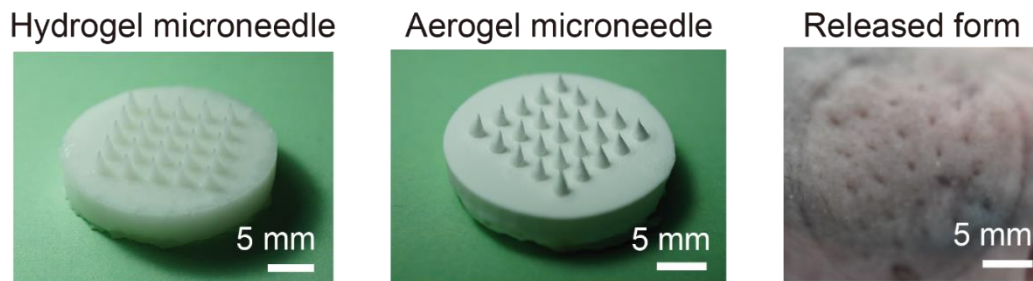
Figure 3-2 The granule-releasing hydrogels can be patterned in hydrogel/aerogel microneedle forms for transdermal delivery of granules. Scale bar, 5 mm.
