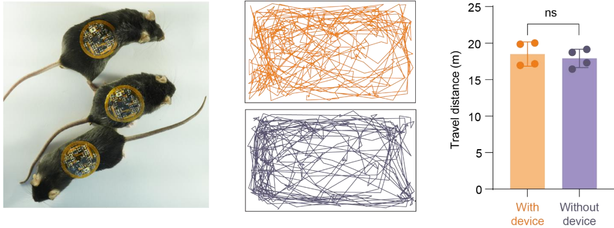
Figure 5-6 Living bioelectronics are lightweight and untethered with cable. (Left) The photograph shows the mice wearing living bioelectronics. (Middle) Representative moving trajectories of mice between the with device and without device group. (Right) The travel distance comparison indicates the living bioelectronics will not interfere with the motion of mice in the cage. Data are presented as mean values \pm SD. n=4 for each group.
