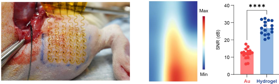
Figure 4-26 Spatial intensity map reveals the sEMG activity across the 15 electrical channels at the rat leg. Size of region: 16 mm (horizontal) \times 12.8 mm (vertical). Comparison of signal-to-noise ratio (SNR) in gold bioelectronics biointerface versus living hydrogel coating indicated that living hydrogels-coated bioelectronics indicates that living hydrogels facilitate electrophysiological recording.
