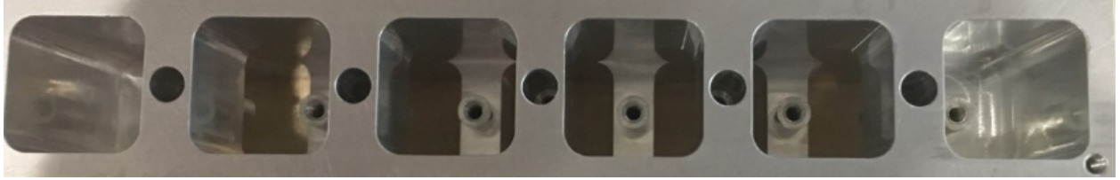
Figure 2.10: Cavities coupled to each other in a 1D lattice. In this particular version, there are posts in both the cavities and the couplers. Tuning the post lengths with a screw allows both the frequency of the cavity and the coupling between sites to be tuned.
