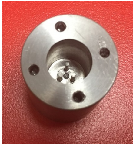
Figure 4.2: Left. Niobium 3 post cavity used to test how to achieve high quality factors with a YIG sphere in the cavity that is biased with a magnetic field. In the center of the 3 posts is a small indentation in which the YIG will rest. Right. Temperature dependence of the quality factor of the niobium cavity without and YIG sphere or field. This set the limit on the maximum quality factors we can obtain in these cavities to \sim 1 million (unless further surface treatment techniques are implemented).
