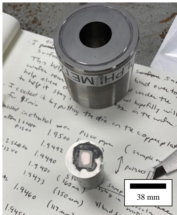
Figure S4. A \text{Mg}_2\text{SiO}_4/\text{MgO} fragment attached to the 38 mm diameter piston of a powder pressing piston-die set. The film is facing the piston, and the Crystalbond applied along the edges of the sample ensured no water reached the film in the center of the sample during wet polishing. Placing the piston in the outer die during hand polishing on SiC paper helped keep the sample flat and level during polishing.
